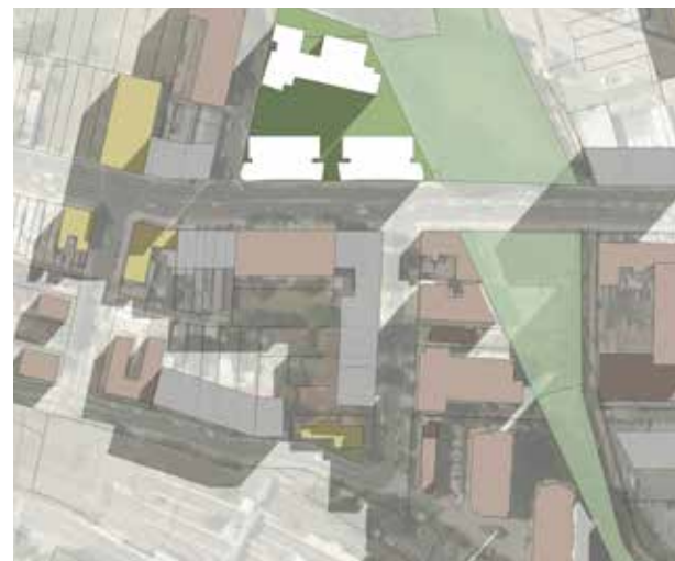
Overshadowing - June 21 at 9am
