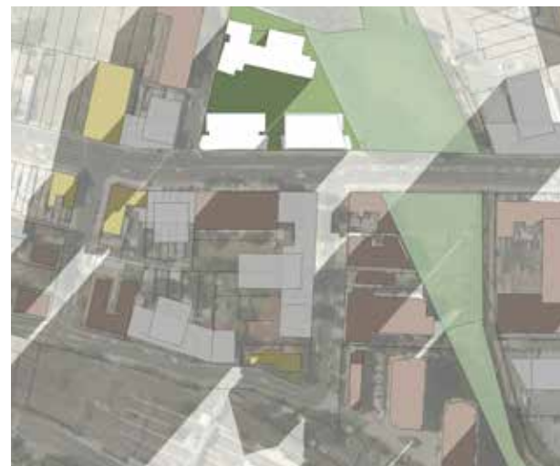
Overshadowing - June 21 at 9am
